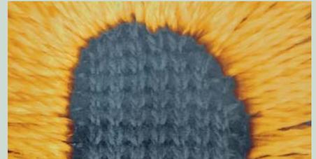
A DB x K5 size 65 with RG-point was used on this fine knitwear, the result is a nice embroidery design without any damage.
